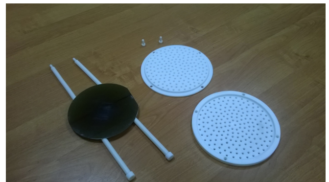
Fig. 1. The cassette for separating a silicon substrate on crystals by liquid etching.
